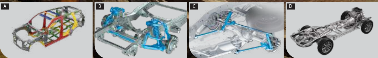
[A] Ultra-High Tensile body structure: Lightweight yet exceptionally strong.
