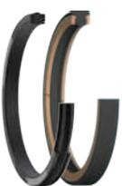
**Locking T-seals** are a patented innovation on the well known T-seal design. Retention features on the backups provide ease of installation without damage. For this reason, locking T-seals are used to replace S-seals, enabling higher pressures and temperatures while reducing damage to metal components.
