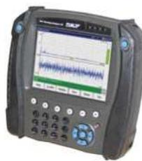
Condition monitoring can be integrated into the bearing to monitor health over its lifetime or provided as a service for trouble-shooting or for confirming condition before/after commissioning. Additionally, because of the slow speed operation of a slewing ring bearing, SKF has developed special vibration analysis techniques for very slow speeds.
