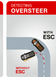
Electronic Stability Control (ESC) detects if the vehicle is under or oversteering.
